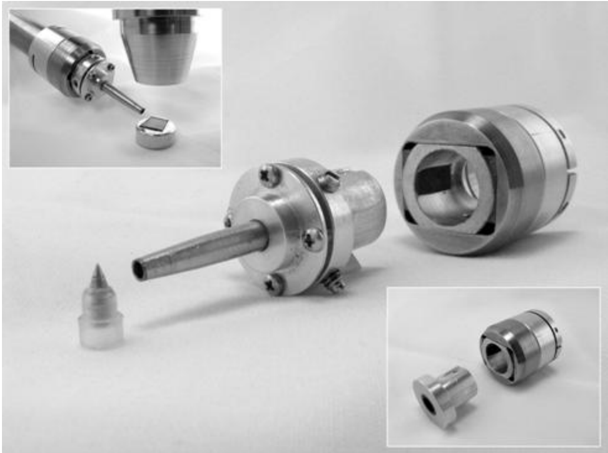
Fig. 2. Parts of the LoMAX. Top left inset shows conceptually how LoMAX attaches to the EDS "snout". Middle shows the LoMAX removable pointer, the optic on its gimbal that slides into the electron trap. Bottom right inset shows the electron trap and the conventional collimator to be used when LoMAX is removed.
